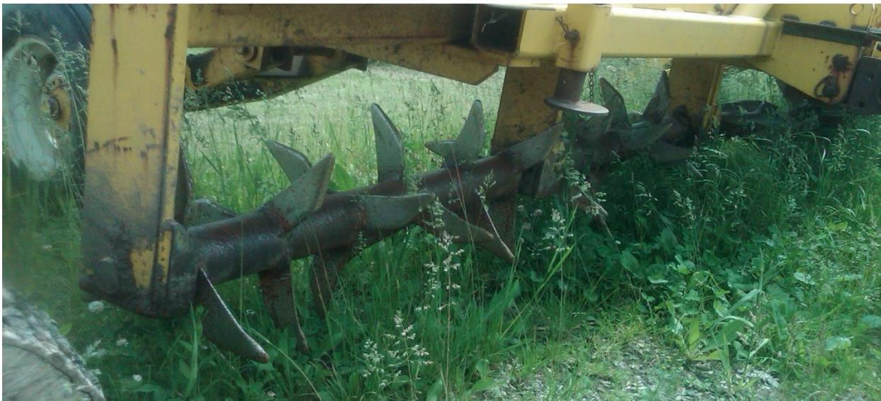
The larger problem with the tine arrangement on this machine lies in the fact that the sequence of the entry events is backwards. The helix should be counter-clockwise but it is clockwise instead (like a regular RH nut). This brand was built with only clockwise helical patterns from 1984 to 2000. The right-hand side of these machines required more ballast to penetrate the soil for this reason and with insufficient ballast the machines would dog-track to the right.
